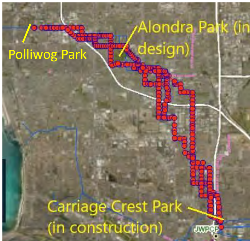
Figure 4-36. Flow Trace in the Sanitary Sewer System from Polliwog Park to the Joint Water Pollution Control Plant
