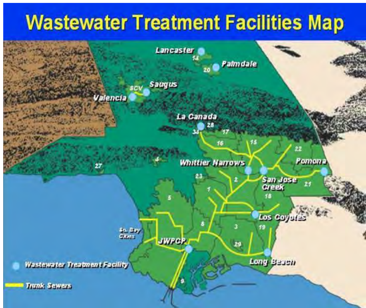
Figure 4-35. Joint Outfall System, Showing 17 Independent Districts, Large Trunk Sewers, 6 Water Reclamation Plants, and the Joint Water Pollution Control Plant
