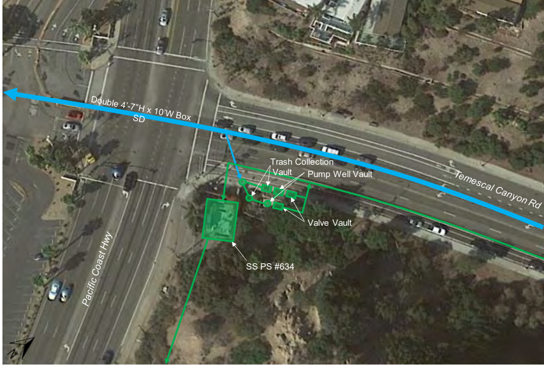
Figure 4-26. Temescal Canyon DWD Location and System Components
