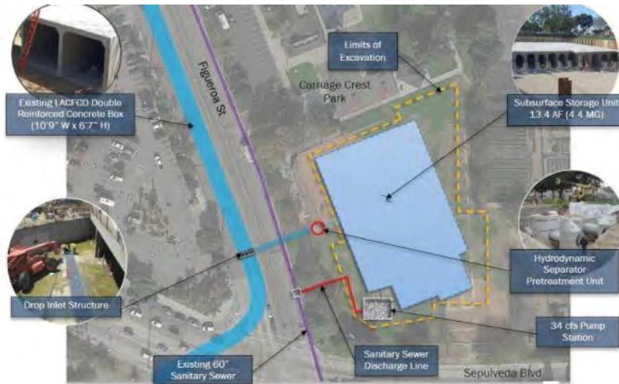
Figure 6-4. Diversion and Storage Features of the Carriage Crest Park Diversion Project
