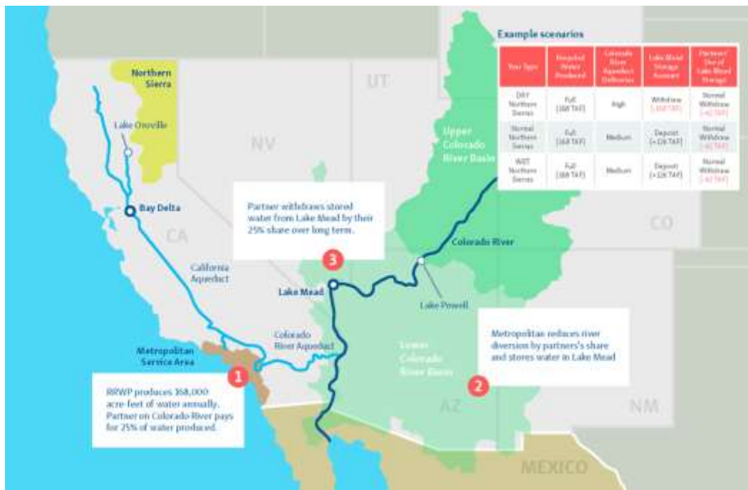
Figure 14: Metropolitan’s Conveyance System and the Regional Purified Water Program Connect Two Critical Watersheds
